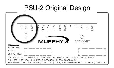
If the PSU-2 matching the above referenced image, is being replaced by the below referenced image, please see the reversed side of this document for wiring the new PSU-2.
